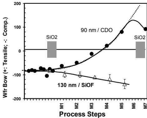
Fig. 4. Wafer level stress as a function of process steps for 90 nm CDO technology and 130 nm SiOF technology. Note that the tensile stress development in CDO stacks is offset by the compressive stress of the oxide layer at the top.
