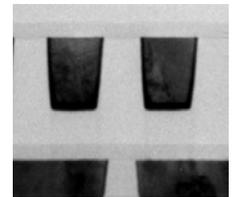
Fig. 2. A TEM image showing simple single ILD/Etch-stop layer stack.
