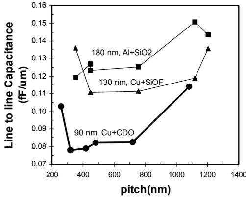
Fig. 7. Line to line capacitance as a function of metal line pitches. 90 nm CDO exhibits 20-25% of capacitance improvement over 130 nm SiOF technology.
