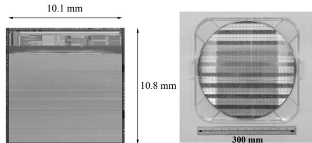
Figs. 10. (left) A single 52 Mbits SRAM chips with 9th technology. (right) A 90 nm technology generation 300 mm wafers with low k ILD and Cu interconnects.
