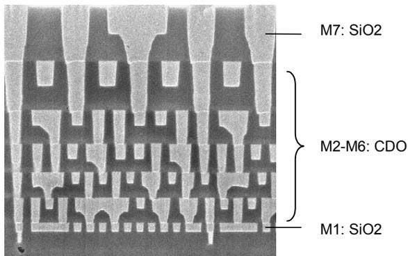
Fig. 1. Cross-sectional SEM photograph showing 7 Cu interconnect layers with either CDO or SiO<sub>2</sub> dielectrics.
