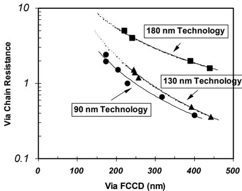
Fig. 5. Normalized via chain resistances as a function of via CDs of various process technologies.
