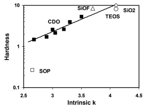
Fig. 3. Hardness vs. intrinsic dielectric constants benchmark for various types of ILD materials.
