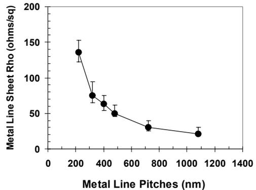
Fig. 6. Metal line sheet rho as a function of metal line pitches. Note the sharp increase when metal line CD below 150 nm.
