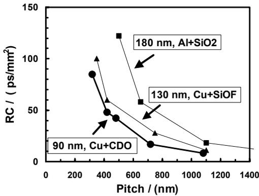
Fig. 8. RC performance trending of 180nm, 130 nm and 90 nm interconnect technology as a function of metal line pitches.
