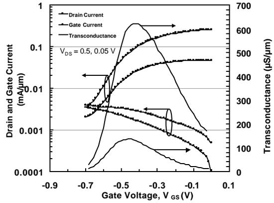
Figure 6. 0.2  $\mu\text{m}$   $L_G$  InSb QW transistor transfer characteristics at 295 K, Type A material,  $L_{DS} = 2 \mu\text{m}$ ,  $W_G = 80 \mu\text{m}$ ,  $V_{DS} = 0.5 \text{ V}$ , 50 mV.
