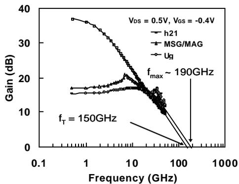
Figure 9. Intrinsic current gain  $|h_{21}|$ , MSG/MAG and Mason's gain  $U_g$  (after de-embedding) versus frequency for 0.2  $\mu\text{m}$  InSb quantum well device with  $V_{DS} = 0.5\text{ V}$  and  $V_{GS} = -0.4\text{ V}$ .
