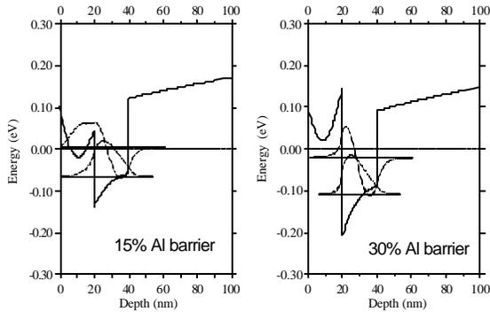
Figure 2. Calculated band structure and Schrödinger-Poisson solution of spatial redistribution of confined carrier population in various sub-bands in the quantum well for 15% and 30% Al percentage barriers.
