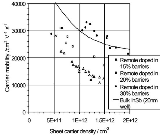
Figure 3. Hall Mobility data on modulation doped 20nm thick InSb quantum wells with 15%, 20% and 30% Al in the  $\text{Al}_x\text{In}_{1-x}\text{Sb}$  barrier layer.
