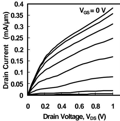
Figure 5. 0.2  $\mu\text{m}$   $L_G$  InSb QW transistor output characteristics at 295 K, Type A material,  $L_{DS} = 2 \mu\text{m}$ ,  $W_G = 80 \mu\text{m}$ ,  $V_{GS} = 0.1 \text{ V/step}$ .
