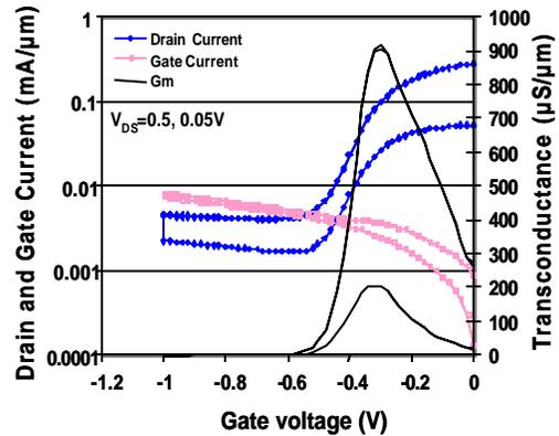
Figure 7. 0.2  $\mu\text{m}$   $L_G$  InSb QW transistor transfer characteristics at 295 K, Type B material,  $L_{DS} = 2 \mu\text{m}$ ,  $W_G = 80 \mu\text{m}$ ,  $V_{DS} = 0.5 \text{ V}$ , 50mV.
