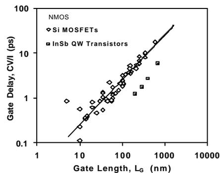
Figure 11. Transistor gate delay (CV/I) vs gate length for InSb QW transistors at  $V_{DS} = 0.5\text{ V}$  bench-marked against state-of-the-art Si nMOS transistors.
