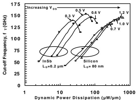
Figure 10. Extrapolated  $f_T$  vs dynamic power dissipation (normalized to transistor width) for InSb QW transistors (solid) for  $L_G = 0.2\text{ }\mu\text{m}$  and state-of-the-art Si nMOS transistors (open) for  $L_G = 80\text{ nm}$ .
