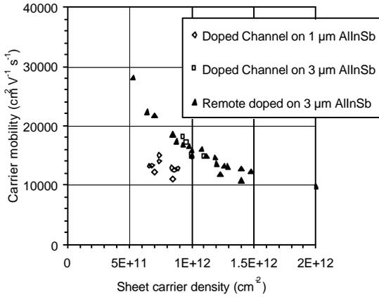
Figure 1. Hall Mobility data on directly doped and modulation doped 20nm thick InSb quantum wells with 15% Al in the  $\text{Al}_x\text{In}_{1-x}\text{Sb}$  barrier layer.
