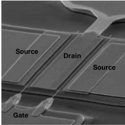
Figure 4. SEM micrograph of a two-finger InSb quantum well transistor with gate air-bridge at the mesa edge.  $L_G = 0.2 \mu\text{m}$ ,  $L_{DS} = 2.0 \mu\text{m}$ .
