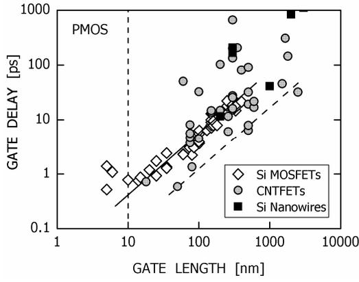
FIGURE 2. Gate delay (intrinsic device speed)  $CV/I$  versus transistor physical gate length  $L_G$  of PMOS devices. The diameters of the CNTs are within the 1.0-2.5 nm range while those of the Si nanowires are within the 4-35 nm range.
