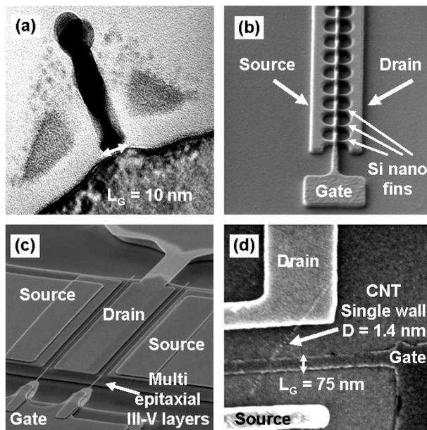
FIGURE 1. TEM cross-section and SEM images of research transistors. (a) Planar Si MOSFET with physical gate length  $L_G = 10$  nm, (b) non-planar Si Tri-gate transistor with multiple Si nano fins, (c) a III-V quantum well FET on a multi-layered epitaxial substrate, and (d) a top-gated CNTFET.
