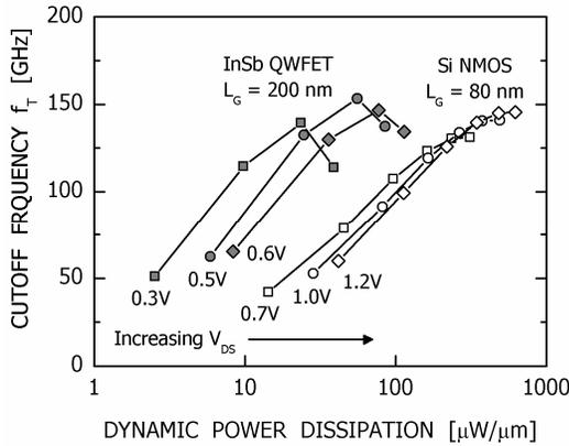
FIGURE 7. Cutoff frequency  $f_T$  versus dynamic power dissipation of an n-channel InSb QWFET with gate length  $L_G = 200$  nm and a Si NMOS with  $L_G = 80$  nm at different values of drain bias  $V_{DS}$ .  $f_T$  is obtained from high-frequency measurement of transistor  $s$ -parameters [20].
