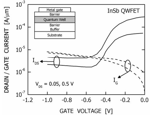
FIGURE 9. Drain current  $I_{DS}$  and gate leakage current  $I_G$  versus gate voltage  $V_{GS}$  of an InSb n-type quantum-well FET (QWFET) with physical gate length  $L_G = 200$  nm. Inset: Schematic of device layers in III-V material-based QWFETs with Schottky metal gates.  $I_G$  is the Schottky gate leakage due to the absence of gate dielectric [20].
