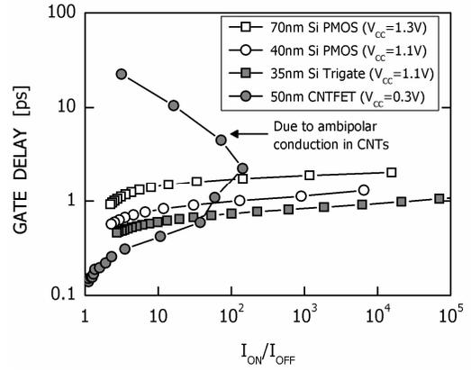
FIGURE 4. Gate delay (intrinsic device speed)  $CV/I$  versus on-to-off state current ratio  $I_{ON}/I_{OFF}$  of Si PMOS transistors with physical gate length  $L_G = 70$  nm at supply voltage  $V_{CC} = 1.3$  V and  $L_G = 40$  nm at  $V_{CC} = 1.1$  V, a Si Trigate PMOS transistor with  $L_G = 35$  nm at  $V_{CC} = 1.1$  V, and a CNT PMOS transistor with  $L_G = 50$  nm at  $V_{CC} = 0.3$  V [17]. The  $I_{ON}/I_{OFF}$  ratio in CNTFETs is limited by the ambipolar conduction.
