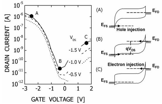
FIGURE 5.  $I_D$ - $V_G$  characteristics of a carbon nanotube PMOS transistor with Pd metal source-drain at different drain biases  $V_{DS}$ , illustrating ambipolar conduction. Pd has a p-type work function with respect to nanotubes. The energy band diagrams exhibit (A) dominant hole injection in the on-state, (B) equal hole and electron injection at the minimum current point, and (C) dominant electron injection in the ambipolar branch.
