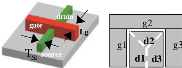
Figure 3. Representation of Tri-gate structure, with cross-section of the gate/channel region
