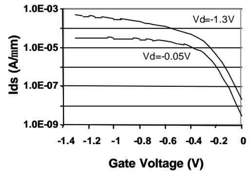
Figure 8. Id-Vg characteristics of a 60nm p-MOS Trigate device
