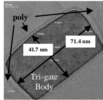
Figure 5. TEM of the silicon body of a Tri-gate device with height 41.7nm and width of 71.4nm
