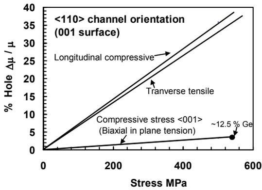
Fig. 1 Hole mobility gain vs. stress from the piezo coefficients in [3].
