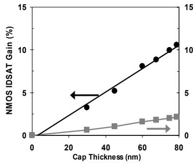
Fig. 7 N & P  $I_{\text{DSAT}}$  vs. nitride capping layer thickness.
