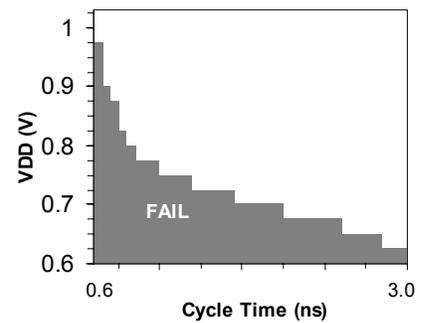
Fig. 11 Schmoof of 50Mb SRAM operating down to  $V_{\text{DD}}=0.65\text{V}$ .
